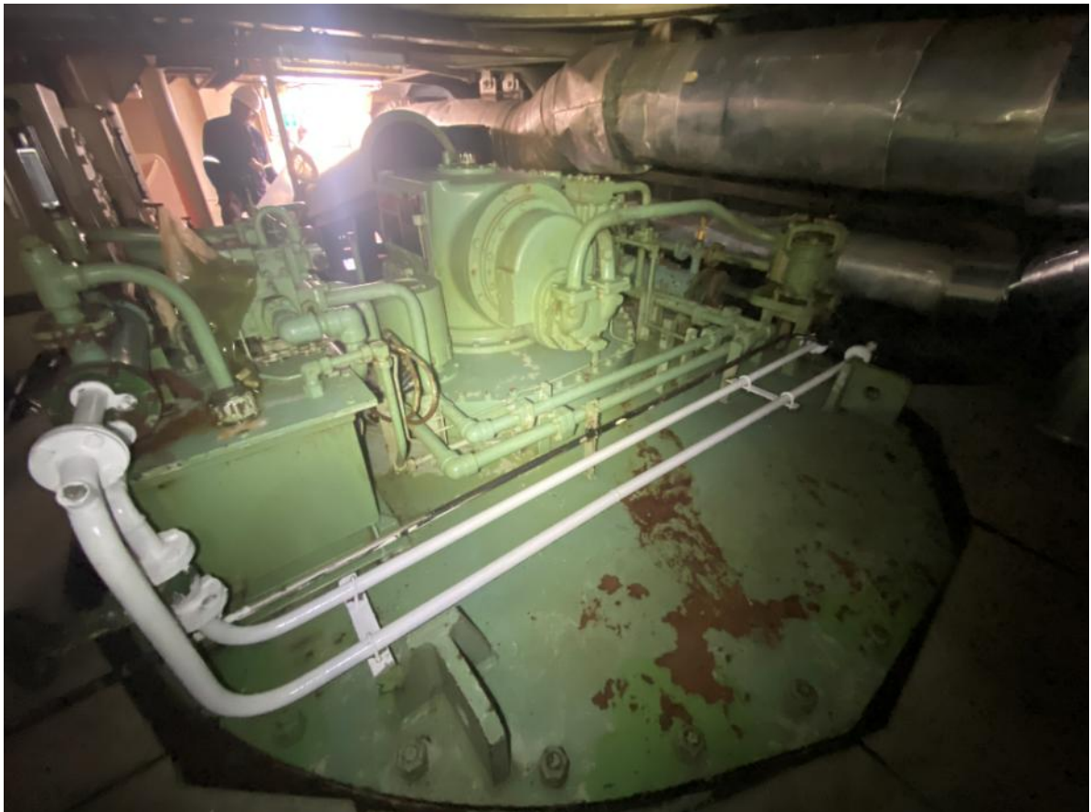
106. Steering room, starboard azimuth transmission and hydraulic pipings.
