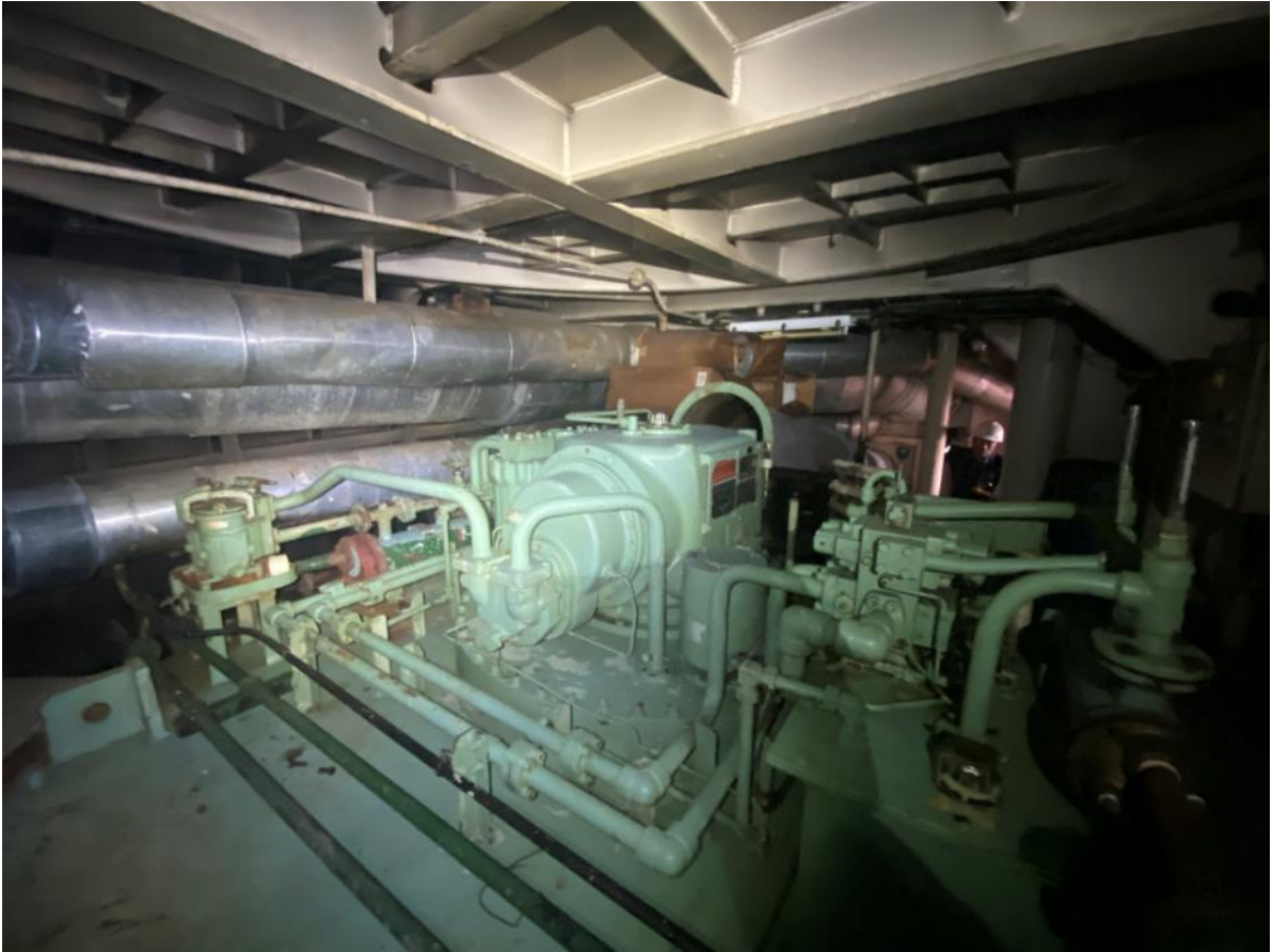
103. Steering room, portside azimuth transmission and hydraulic pipings.
