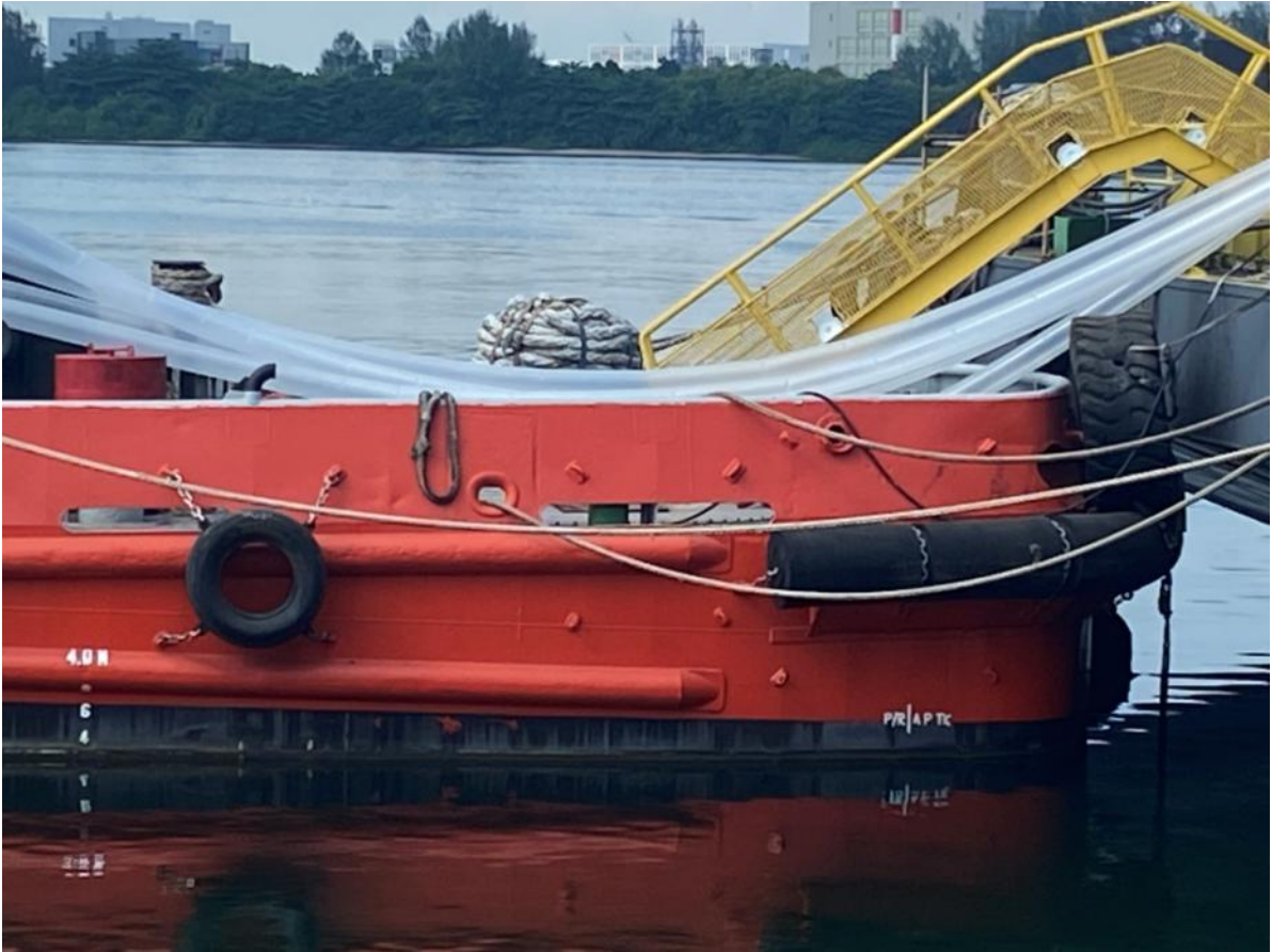
005. Aft fenders replaced.
