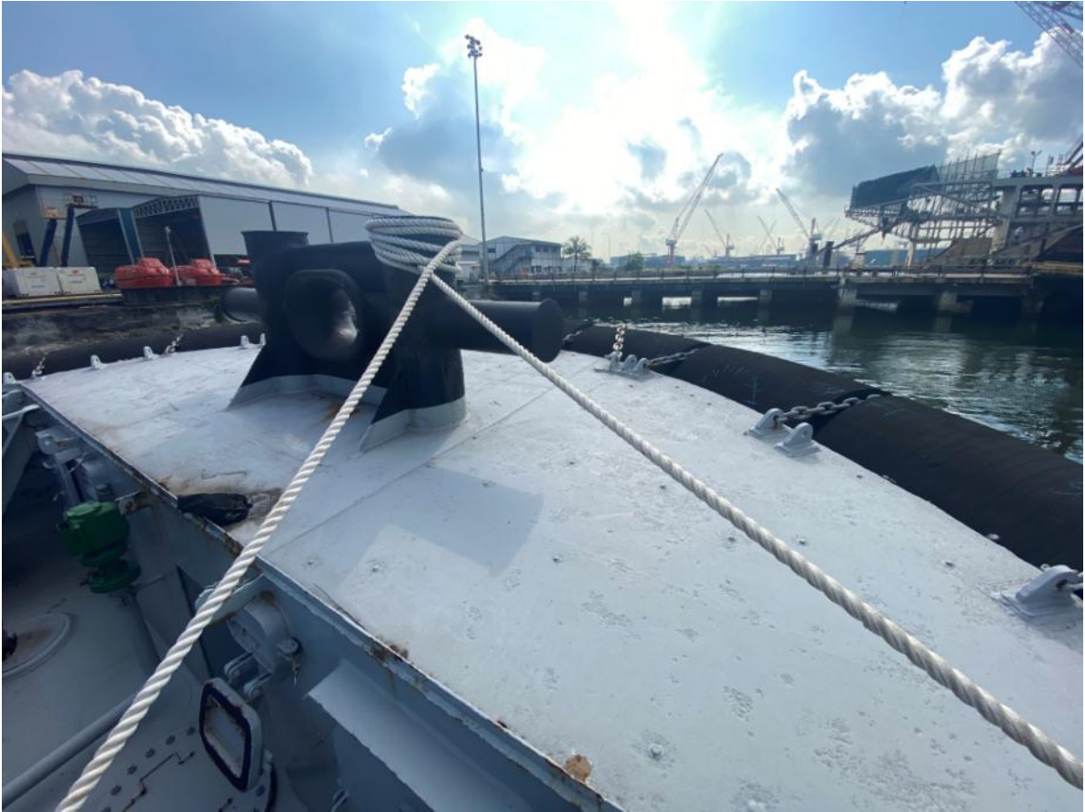
007. Fore-end of the vessel with towing staple well coated.
