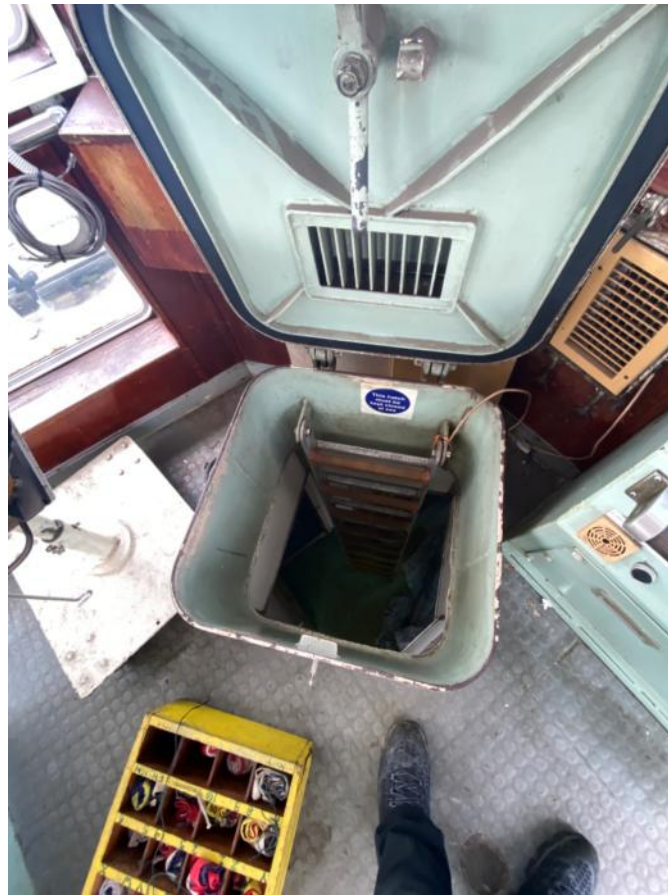
035. Access hatch into crew accommodation space.
