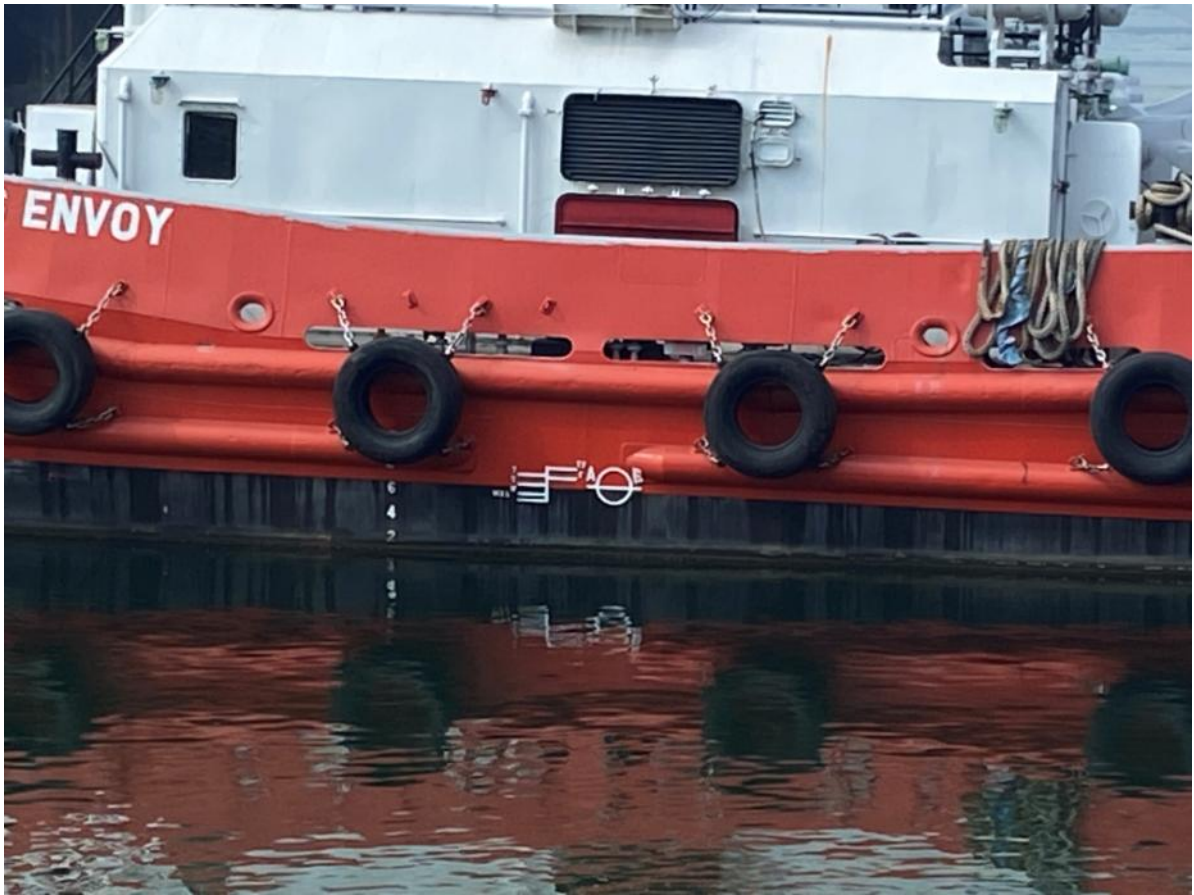
003. Plimsoll mark and hull general coating appeared in good condition.
